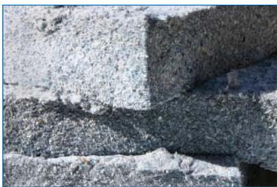
*Cotton batt insulation made from recycled denim.*
